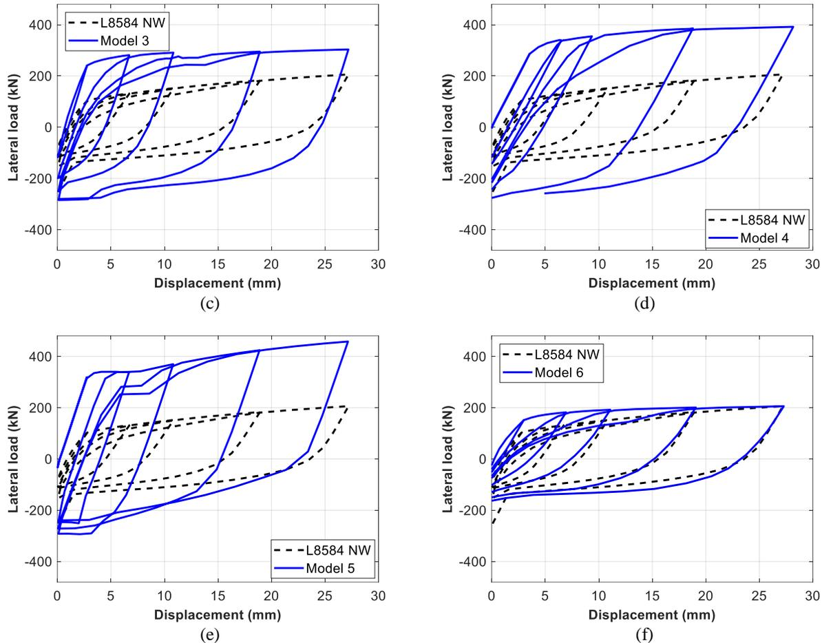
Figure 4. (a-f) Load-deflection behavior of model 1-6
