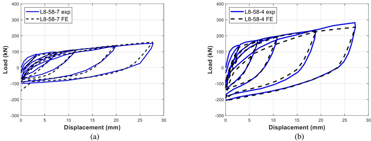
Figure 2. Comparison of the load-deformation behavior between experimental and FE model: (a) L8-58-7, and (b) L8-58-4
